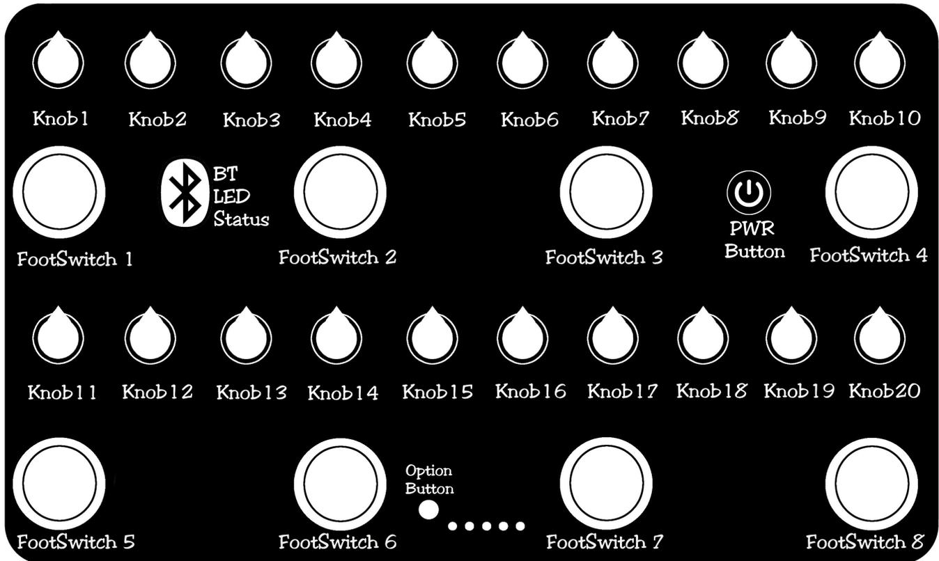
**Footswitch LED's** - Every footswitch has it's own LED, which indicates footswitch being pressed. You are able to set different messages on "LED on" and "LED off" actions. Device is able to receive MIDI messages, so if you receive same message, programmed to footswitch - LED will light up or light down.
